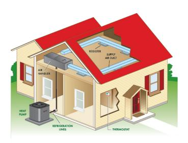
**Emergency Heating:** Should the heat pump fail, activate the emergency switch on the thermo¬stat. The red light indicates that it is on. This will stop the heat pump from operating and will provide supplemental heat until the HVAC contractor arrives.
